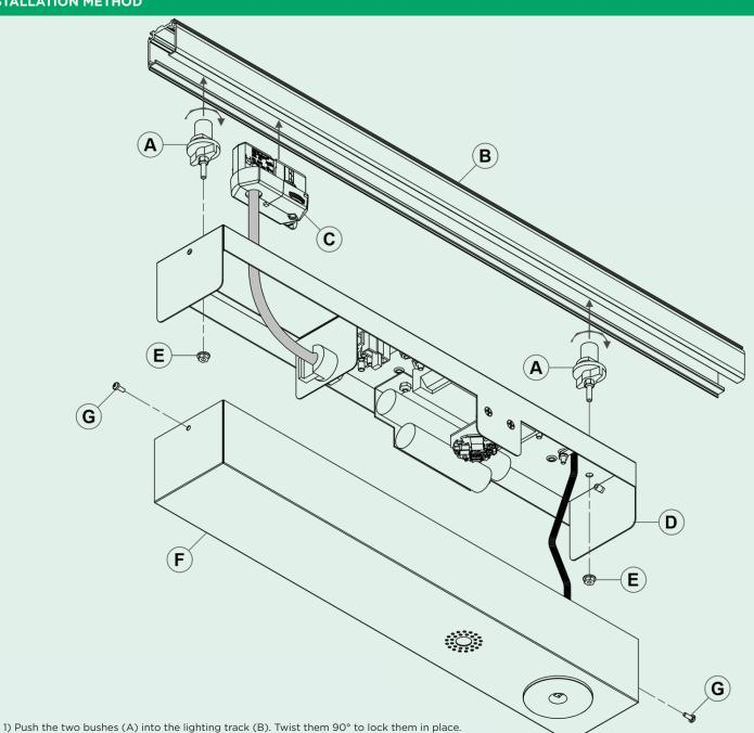
2) Set the circuit selector switch, on the track adaptor (C), to the common permanent (un-switched) live feed that has been chosen for the use with the emergency lighting. This feed must come from the samelocal sub-circuit as the local mains lighting.
