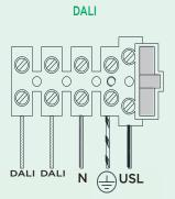
BASIC INSULATION IS MAINTAINED BETWEEN THE LV SUPPLY AND CONTROL CONDUCTORS ON THIS LUMINAIRE.
