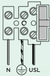
BASIC INSULATION IS MAINTAINED BETWEEN THE LV SUPPLY AND CONTROL CONDUCTORS ON THIS LUMINAIRE.
