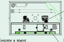
WIRE INTO THE REFLECTOR TERMINAL BLOCK USING THE WIRES FROM "1" ENSURING POLARITY. CONNECT THE EARTH CABLE INTO THE EARTH TERMINAL IN THE FUSED TERMINAL BLOCK
