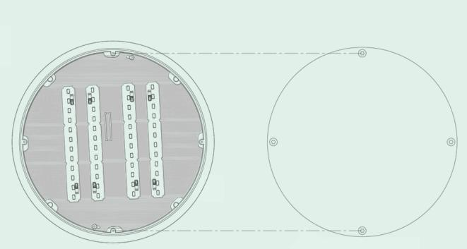
COVER SECURED WITH 4 X SECURITY SCREWS
