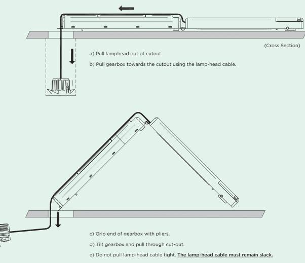
f) If the lamp-head cable is pulled tight, the gearbox will not bend, and it will be very hard to remove from from the ceiling without causing damage.
