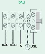
BASIC INSULATION IS MAINTAINED BETWEEN THE LV SUPPLY AND CONTROL CONDUCTORS ON THIS LUMINAIRE.
