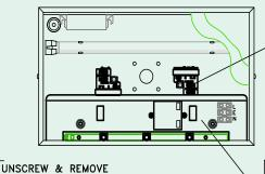
WIRE INTO THE REFLECTOR TERMINAL BLOCK USING THE WIRES FROM "1" ENSURING POLARITY. CONNECT THE EARTH CABLE INTO THE EARTH TERMINAL IN THE FUSED TERMINAL BLOCK
