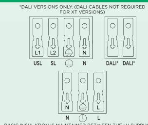
BASIC INSULATION IS MAINTAINED BETWEEN THE LV SUPPLY AND CONTROL CONDUCTORS ON THIS LUMINAIRE.
