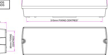
\*FIXING HOLES Ø4mm
