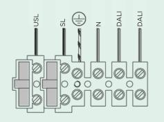
BASIC INSULATION IS MAINTAINED BETWEEN THE LV SUPPLY AND CONTROL CONDUCTORS ON THIS LUMINAIRE.
