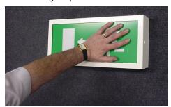
**D.** Gently pull back on tool to remove frame, leaving legend free. Lift legend to access gear tray.
