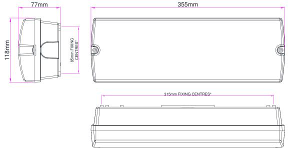
\*FIXING HOLES Ø4mm
